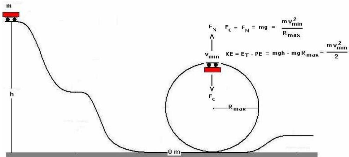
A roller coaster of mass  $m$  at rest at the top of a frictionless roller coaster track of height  $h$  descends to base level and then enters an inverted circular loop. Derive the equations for calculating the maximum permissible radius [ $R_{\max}$ ] of the inverted circular loop in order for the roller coaster to remain on the track and completely transit the loop.
